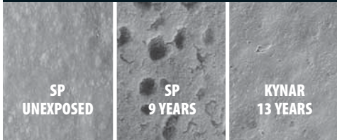
Photomicrographs (enlarged 500X) show comparative film erosion. The left photo shows silicone polyester before it was exposed to the elements. In just nine years, the finish is crumbling in the center photo, while the Kynar 500 sample still looks great after 13 years of exposure.
