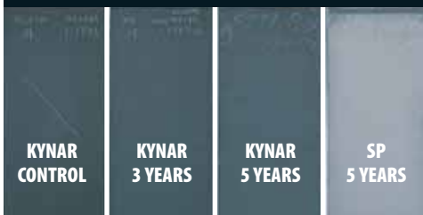
Examine the difference in performance of Kynar 500 when compared to silicone polyester. When exposed to the sun's UV radiation for 3-5 years, Kynar 500 samples show almost no change. The silicone polyester sample shows severe fade and chalk... the whole system is disintegrating.
