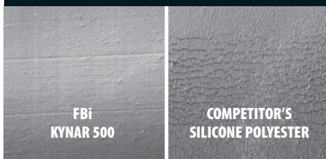
These photos show metal building panels which were identically roll formed (the process used to create ribs in the panels). They show the finish at an outward bending ridge in the same area of each panel. Notice the cracks which formed on the competitor's product because of poor flexibility. Over time, these cracks will allow moisture to reach the steel substrate. Rust and corrosion are inevitable.
