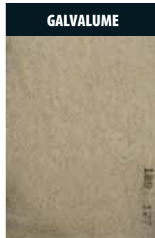
The Galvalume sheet panel continues to perform well after the same 23-year exposure.
