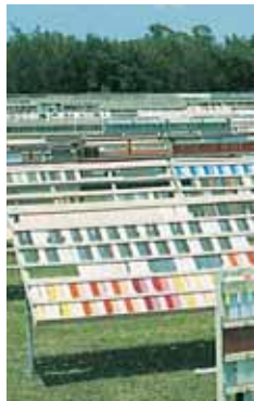
FBI paint systems are exposed to severe Florida weather for years to insure the quality of finish on your building.
